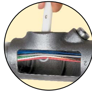
The large hook on Tool #3 quickly lifts all the conductors.
