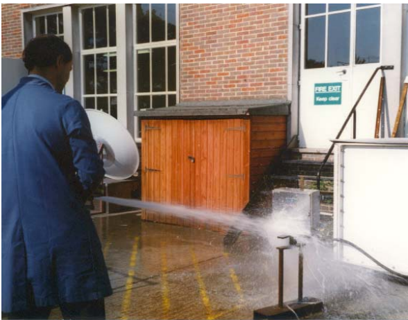
Marine ratings undergo extreme hose and deluge tests.
