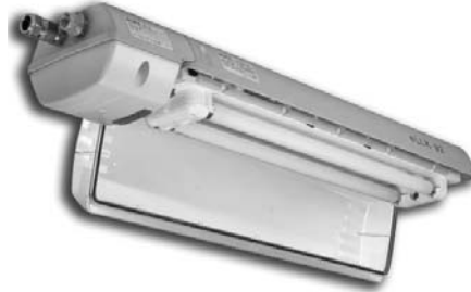
The Ex-q concept was originally used for the electronic ballast in the SpecOne eLLK fluorescent luminaires. (The ballast was redesigned in 1992 to the Ex-d design.) If these devices fail, they are replaced “like for like” from the original manufacturer as a certified spare part. The user cannot repair them..
