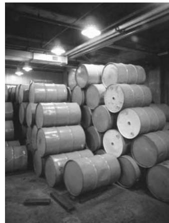
Areas where volatile liquids are stored are normally classified as Zone 2 or Division 2.
