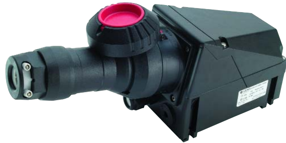
The Cooper Crouse-Hinds Zone 1 plug will operate the Zone 1, Zone 2 and ordinary location receptacle. The Zone 2 and ordinary plugs will not operate the Zone 1 receptacle. This is to prevent non-rated portable equipment from being used in a classified location.
