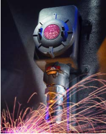
The FSQ is available in for Class I, Division 1 areas in 30, 60 & 100 amps. Rotating the plug after insertion activates this switch and locks the plug in place.
