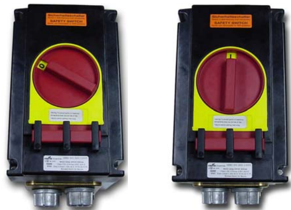
Each Cooper Crouse-Hinds SpecOne™ disconnect switch has a position ring with OFF-ON or (O-I) defined switch positions. The contact blocks can have optional auxiliary contacts for wiring to separate lamps or other devices for local or remote indication.
